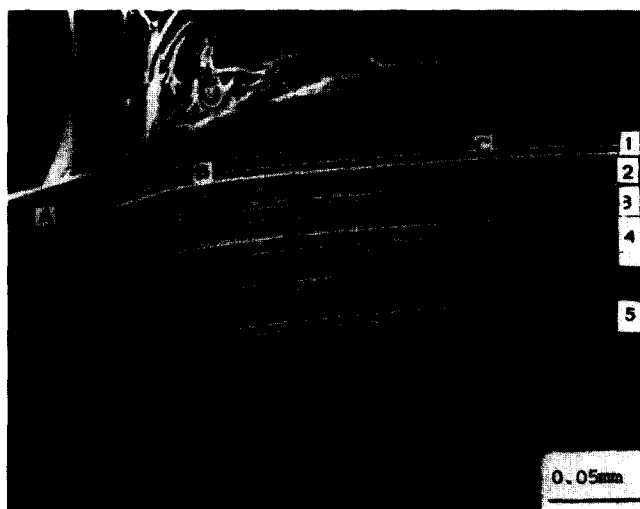
Figure 9 SEM micrograph for a specimen whose notch was opened to 144 \mu\text{m} at room temperature for a craze originally formed at 80°C with a 86 \mu\text{m} notch opening
